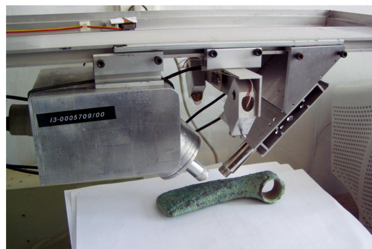
A detail, on the left is the source of X-rays, on the right is detector and in the middle is examined object.
